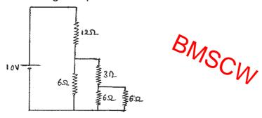
10. Using mesh current method, find the branch currents for the following circuit.
