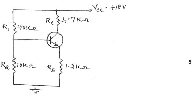
12. For the circuit shown, calculate the values of  $A_V$  and  $r_{out}$ . Given  $V_{BE} = 0.7 \text{ V}$  and  $\beta = 100$ .
